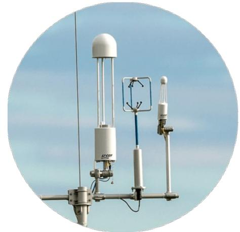
Figure 5: A typical multi-sensor eddy covariance system
