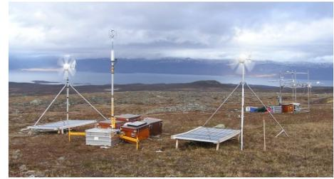
Figure 7: Combined Eddy Covariance and Micrometeorological Station near Abisko, northern Sweden
