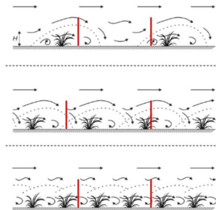
Figure 1: Wind flow over various vegetation densities. Red lines represent an EC system on top of support pole.
