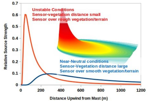
Figure 3: Source area curves upwind of sensor mast
