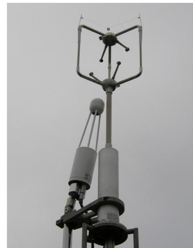
Figure 6: Solent R3 Sonic Anemometer-Licor 7500 IRGA System
